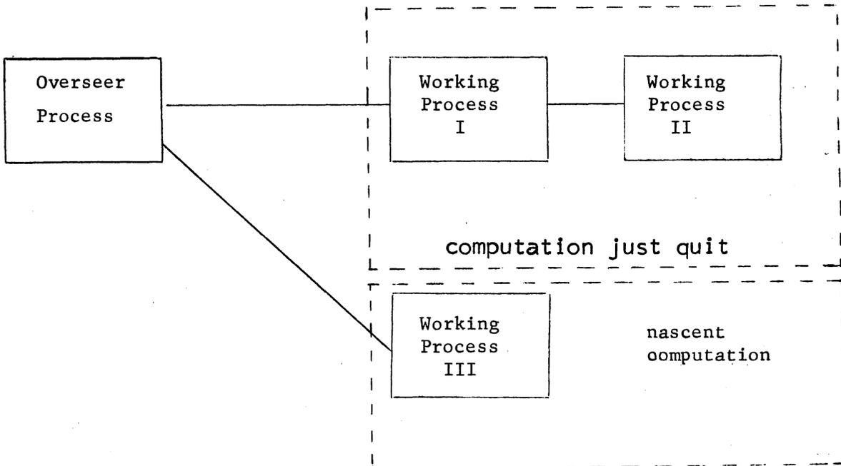
In this example, a user was executing a command which created another process for concurrent processing. Then he pressed the quit button at his console. Now if he types the start command the two processes executing his former computation will be restarted and Working Process III destroyed. Otherwise, Working Processes I and II will be destroyed and he will continue with the fresh computation in Working Process III.
