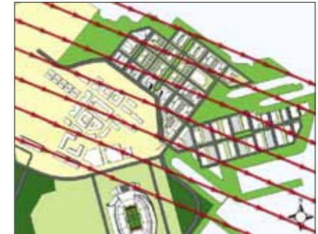
Street and block pattern oriented at 45° to prevailing winds at Hunters Point
