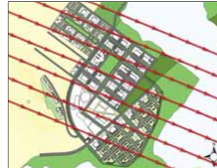
Street and block pattern oriented at 45° to prevailing winds at Candlestick Point
