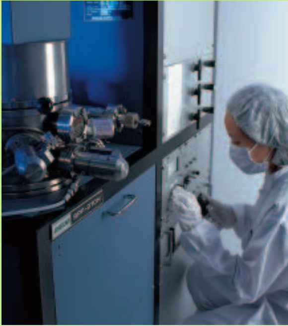
Deposition of Silicon-Germanium thin film using an Argon Plasma RF Sputterer.
