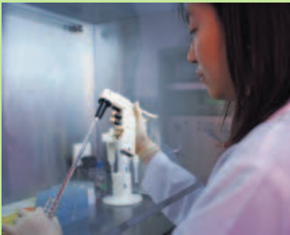
Handling of an Electronic Pipettor in a Biosafety Cabinet.
