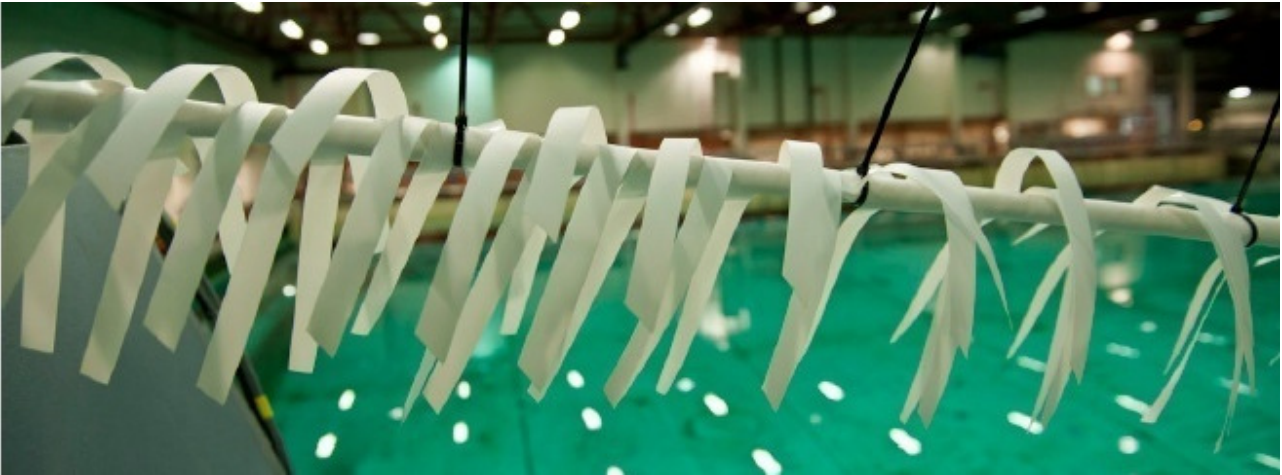
Figure 2: Small pipe covered with wrapping ribbon fairings
