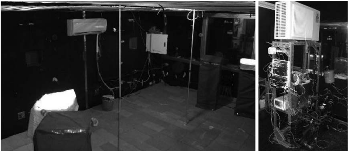
Figure 3. Left: Test office chamber with concrete radiant floor, simulated internal loads, and a conventional split-system air conditioner indoor unit. Right: Low-lift chiller in the climate chamber.
