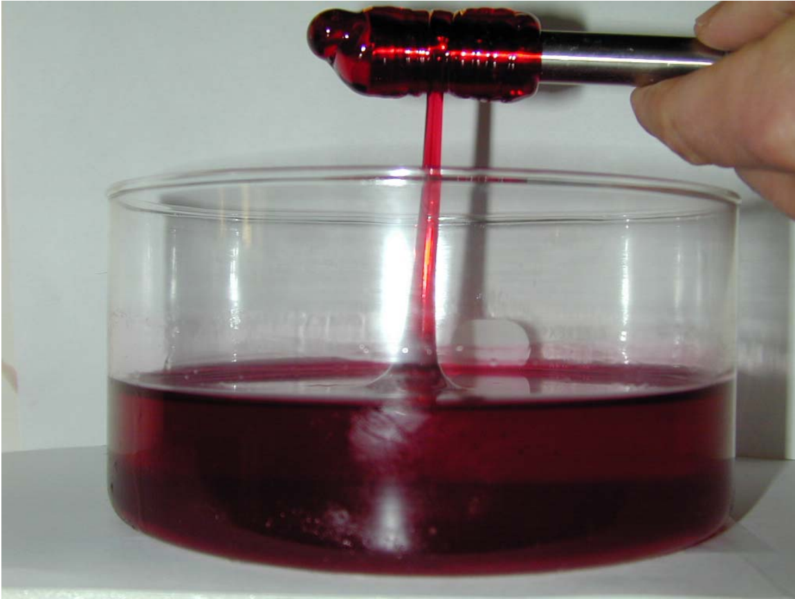
Figure 1.2 The tubeless siphon. In the images above, a dyed polybutene Boger fluid is wound upwards onto a rotating spool.
