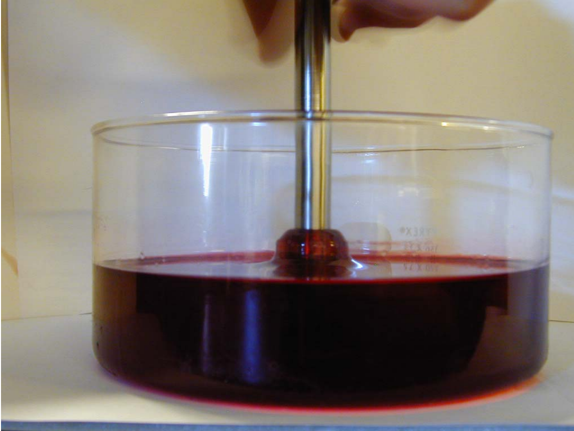
Figure 1.3 The rod-climbing effect. In the images above, a dyed polybutene fluid is stirred with a rotating rod. The streamlines contract around the rod and the fluid ‘climbs’ the rod.
