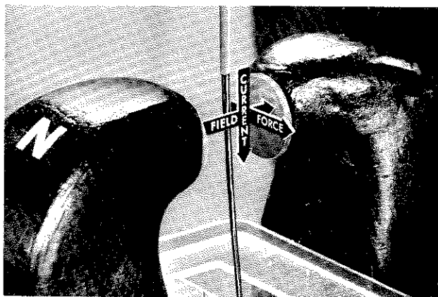
1. A vertical mercury jet carrying a vertical electric current \mathbf{j} in a horizontal magnetic field \mathbf{B} is deflected by the \mathbf{j} \times \mathbf{B} force.
