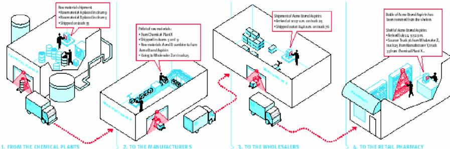
Chemical plants create raw materials and place them into drums. Each drum is uniquely numbered and tagged with RFID tags so the EPCTM Network can track them to the manufacturer. From this point on, the history of all raw materials is recorded in the EPCTM Network.
