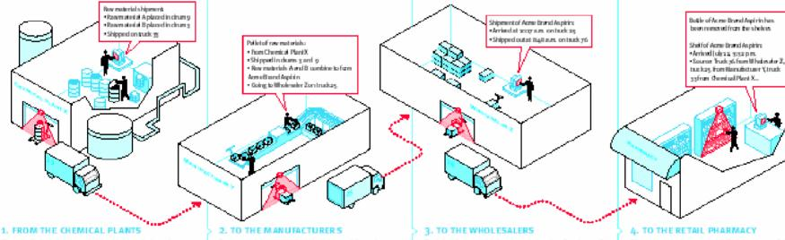
Chemical plants create raw materials and place them into drums. Each drum is uniquely numbered and tagged with RFD tags so the EPC™ Network can track them to the manufacturer. From this point on, the history of all raw materials is recorded in the EPCTM Network.
