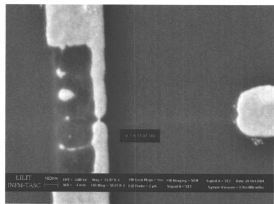
FIG. 2. SEM images of pattern obtained using different FIB milling time; (a) gaps between 20 nm using 3 s, 10 nm (b) using 2 s and those with a thin gold wire branching the gap (c), using just 1 s. All 3 types of gaps were obtained with a good repeatability.
