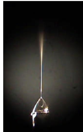
Figure 5: Cone-jet structure in the laboratory. The liquid used had low conductivity, which allowed the jet to be large enough to be visible. With more concentrated solutions, the jet diameter is smaller than the wavelength of light and becomes invisible.
