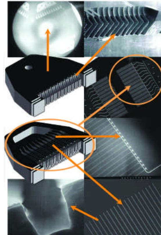
**Figure 8:** Fabrication details in the linear array engine. The top left panel shows the wafer with several engines after bonding the two halves and annealing.
