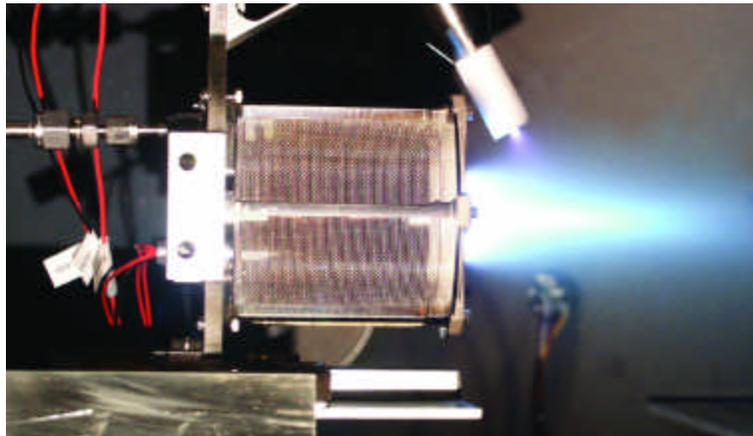
**Figure 2:** A 200W Hall thruster (courtesy Busek Co. Inc.) in the 1.5X1.5 m vacuum chamber at the SPL. The blue light is mainly from excited Xe ions in the plume. The device at the top is the neutralizing hollow cathode.
