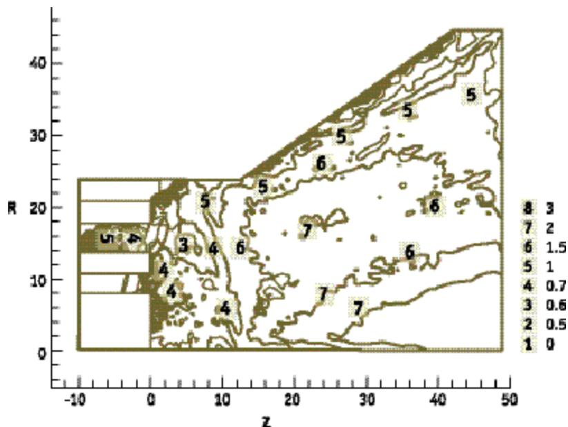
Figure 3: Computed contours of the ratio of parallel to perpendicular electron temperature in a Hall thruster. Deviations from unity indicate the anisotropy due to the strong magnetic field.
