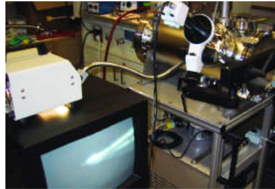
**Figure 6:** The SPL small vacuum facility for colloid research. The microscope display is showing the tip of a cone-jet emitter in operation.
