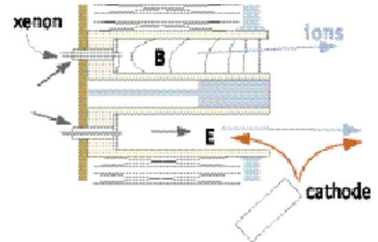
**Figure 1:** Schematic of a Hall thruster. The annular channel is ceramic lined. A plasma forms near the exit plane, where the magnetic field,  $B$ , is maximum. Ions accelerate electrostatically in an electron-neutralized background, and no grids are necessary.
