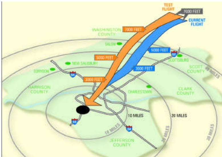
Standard flight paths at Louisville (blue) involve a series of staggered descents producing significant noise from multiple thrust increases and landing-configured aircraft systems. The test path (orange) keeps aircraft higher, longer. (Drawing adapted from a Covington Journal Illustration by Mike Covington)
