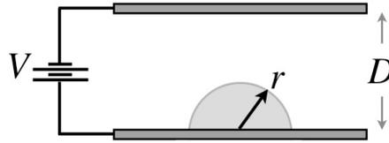
This setup is typical for generating the electrostatic liquid instability that forms Taylor cones when the electric pressure balances the liquid surface tension at some critical voltage  $V_0$ .
