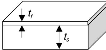
The sketch above represents a film barrier coating perfectly joined to the surface of a planar substrate, having thicknesses  $t_f$  and  $t_s$ , respectively. Both materials are isotropic.
