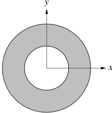
$$\begin{aligned} \nabla^2 \phi &= 0 \\ \nabla \phi \cdot \mathbf{n} &= \sigma(x, y) && \text{(on outer boundary)} \\ \phi &= 0 && \text{(on inner boundary)} \end{aligned}$$
