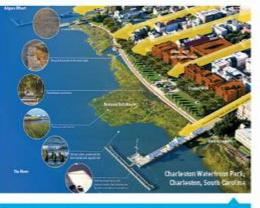
Crushed stonedust, preserved pier piles, local brick, marine wood, and recyled granite are utilized in the waterfront :
