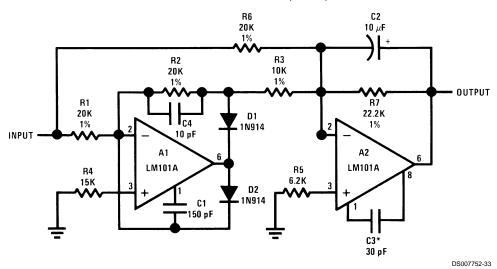
Note 8: Feedforward compensation can be used to make a fast full wave rectifier without a filter.
