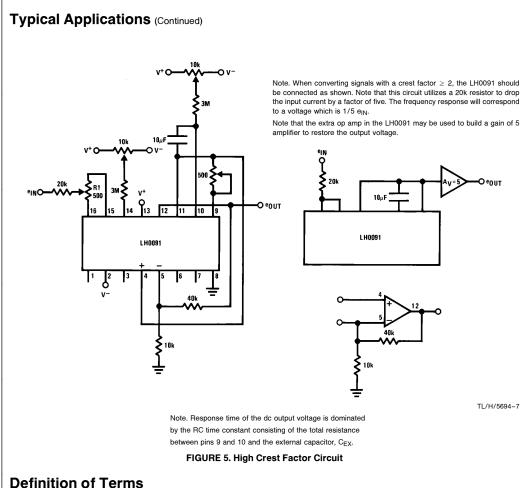
True rms to dc Converter: A device which converts any signal (ac, dc, ac + dc) to the dc equivalent of the rms value.
