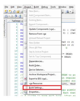
Within the build settings, the particular setting is found under "Linker". Setting the highlighted "Custom Linker Script" path to the actual, absolute, path of your custom linker script will properly include it.
