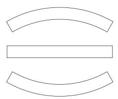
The block is made of springs, and it acts like a big spring. The middle position is the equilibrium position, when the block has zero potential energy and maximum kinetic energy. The potential energy is stored in stretching and compressing the bonds. Imagine deforming the block into a shape like the top shape. Since the block is a big spring, to produce the vertical deflection y requires an energy  $E \sim ky^2$ , where k is the stiffness of the block.
