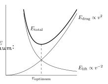
so that its cruising speed is its minimum-energy speed. So at takeoff and landing, when its speed is much less than the minimum-energy speed, a plane requires a lot of power to stay aloft, which is one reason that the engines are so loud at takeoff and landing (another reason is probably that the engine noise reflects off the ground and back to the plane).
