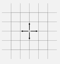
By symmetry, removing 1 A produces 1/4 A in each coordinate direction, flowing toward the terminal. Let's call this terminal the negative terminal. So removing 1 A produces 1/4 A through the selected resistor, flowing toward the negative terminal. Equivalently, it produces 1/4 A flowing away from the positive terminal.
