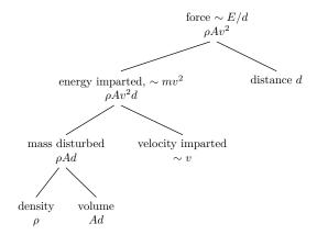
The result that  $F_{\rm drag} \sim \rho v^2 A$  is enough to predict the result of the cone experiment. The cones reach terminal velocity quickly – a result discussed later in the book in **Part 3** – so the relevant quantity in finding the fall time is the terminal velocity. From the drag-force formula, the terminal velocity is
