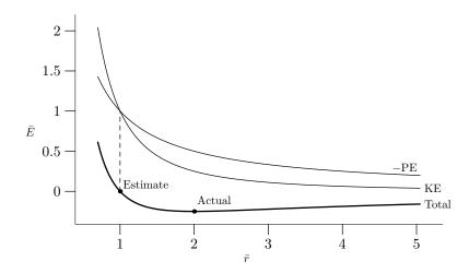
Calculus (differentiation) locates this minimum-energy  $\bar{r}$  at  $\bar{r}_{min} = 2$ . An alternative method is **cheap minimization**: When two terms compete, the minimum occurs when the terms are roughly equal. This method of minimization is familiar from **Section 6.2.2**.
