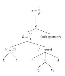
sketching the solution tree, leaving  $\rho$  as depending on R plus geometry. We can find R by placing a voltage V across a block of seawater and measuring the current I; then R = V/I.
