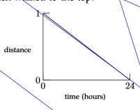
And this diagram shows the upward and downward schedules on the same diagram. Something interesting happens: The curves intersect! The intersection point gives the time and location where the upward and downward schedules landed on the same point at the same time of day (but on separate days).
