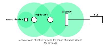
rupted by a wall or a floor, that range will decrease to 20 feet. BLE repeaters are extremely cheap (ten dollars per repeater) and draw very little power from their built-in battery. For the purposes of this project, you can assume that the batteries never need to be replaced.
