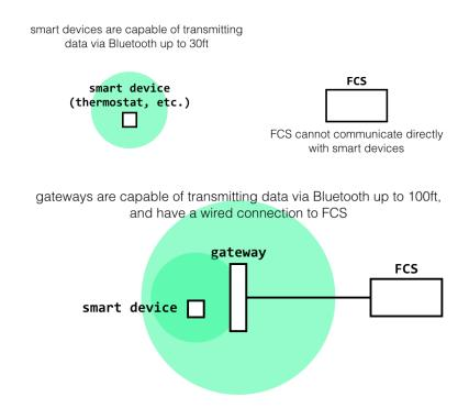
In addition to acting as a bridge between Bluetooth components and the rest of the Internet, gateways can send transmit data via Bluetooth with a range of 100 feet and have 32 GB of persistent storage. If a gateway has to transmit through a wall or floor, its range will decrease by about ten feet for each impediment (e.g., if the signal needs to pass through a single wall, it will have a transmission range of 90 feet).
