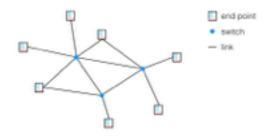
Typically we'll refer to machines such as your computer as "endpoints", to differentiate them from switches. Usually, endpoints initiate the sending of data, and data is sent to them; switches help move data through the network. As you can see, data from multiple different endpoints might pass through a single switch.
